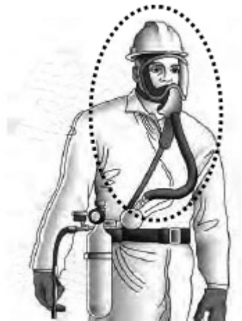
Supplied air respirator with full face mask
