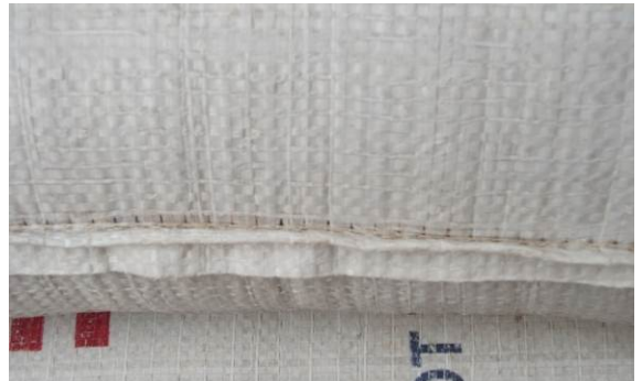
Photo no. 4: Polypropylene Bag with Wheat Showing Gaps Near the Stitches. (Insects can easily enter through these openings (Adama, Ethiopia)
